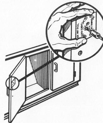
Measure door thickness, then subtract  $3/16"$ . Position **drill depth gauge** on bit and move it the required distance from the tip so hole drilled will be within  $3/16"$  of cabinet door front. Drill into "7MM HOLE" location on guide.
