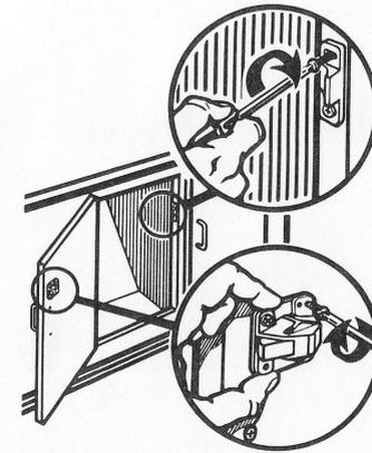
Match striking plate over 2 locations marked during Step 1. Use screws and install loosely so slot adjustment can be made later. Match TOT-LOK Assembly into 7mm holes (install Plunger/Slug if necessary), align over 4 marks (from Step 2) and screw in place with four  $1/2"$  screws. A pair of auxiliary holes are provided for variations in door panels. Assure proper function prior to closing. Note proper position of striking plate and screw it down tight.
