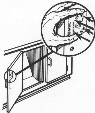
Close door firmly on foam tape. This will transfer guide to exact location on inside of door (or drawer). Open door, hold guide down, and mark 4 screw locations for lock installation (4 arrows).
