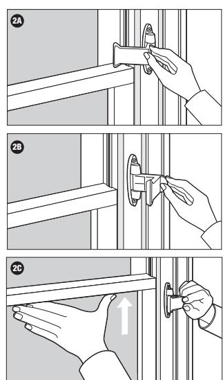
NOTE: Some side window sashes will be narrow and Window Stop will rest on glass when window is open more than 4". When this is the case, pull arm away from window when closing. Once window is closed, release arm and Window Stop will automatically reset.
