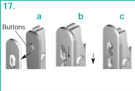
Center buttons of assembly with wall plate holes (17. a). When aligned, push buttons through holes and slide down to lock (17. b & c).
