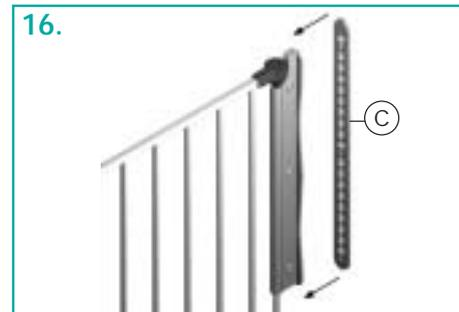
Fasten wall plate (C) onto assembly. See steps 17. a, b and c.
