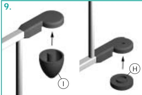
Remove hinge cap (H) from bottom of original end section. A screwdriver may be needed to pry it off. Place under bottom hinge. Remove plastic cone from under top hinge of original end section. Install cone (I) under top hinge of new end section.
