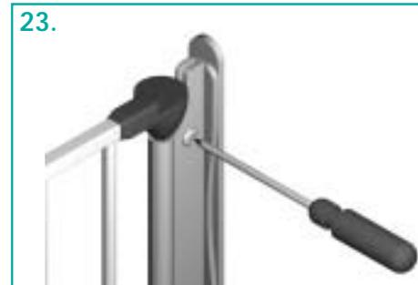
Tighten 3 sets of assembly screws and nuts.
