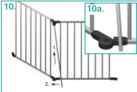
Reinstall a removable, vertical bar. Insert bar by pressing it into upper hinge cone, while sliding bar into groove of lower hinge. Spring in cone will make bar lock in place. Proceed to "Installation" steps 13 to 23.
