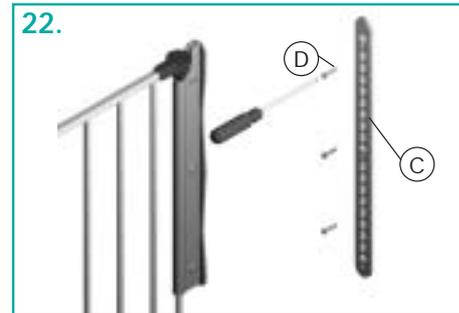
**Note:** Screws provided are for mounting directly into wood. If mounting into brick, drywall or other surfaces, use appropriate hardware.
