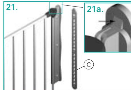
Remove wall plate (C) from assembly by pressing locking tab (21a.) and lifting it off.
