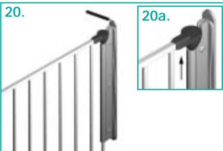
Slide the assembly as close to cone as possible (20a.). With a pencil, outline assembly on mounting surface.
